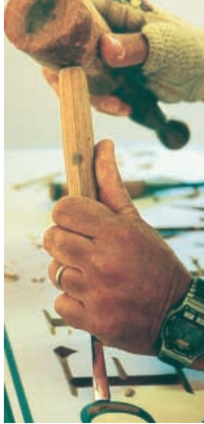
For curved strokes, I use a gouge—a chisel with a curved blade.
