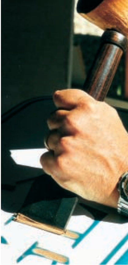
The straight strokes are cut at an approximately 110° angle, using assorted flat chisels.
