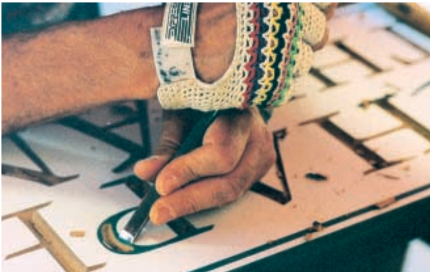
I wear a bicycle glove on my right hand to protect my palm while pushing on the gouge. I use my left hand to position and guide the gouge.
