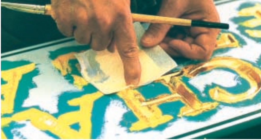
Gilding is easy. Position the tissue of gold over the sized letter and press on the back of the tissue, forcing the gold into the letter.
