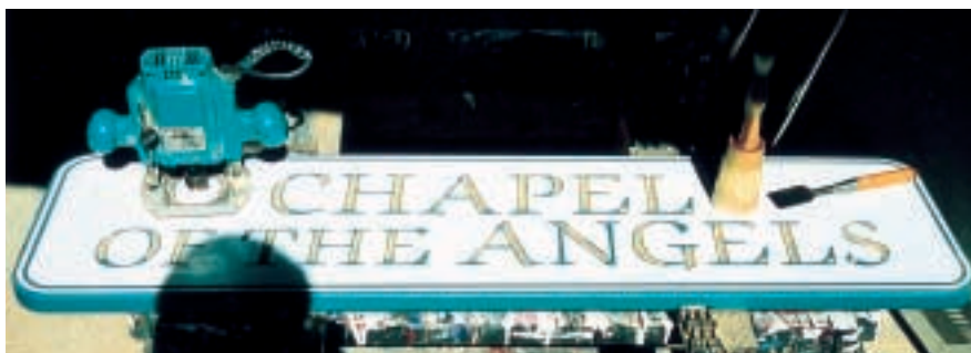
After applying a computer-cut mask to the painted panel, I use a V-bit in a router to cut the wide strokes.
